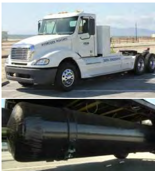
Vision's Tyrano truck uses 6,250-psi Worthington Type III fuel cylinders
