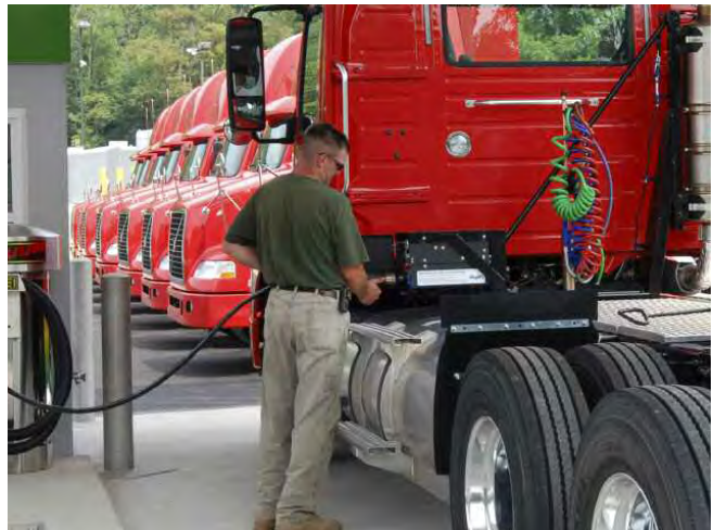
Note diesel-look alike CNG fuel assembly by Agility Fuel Systems
