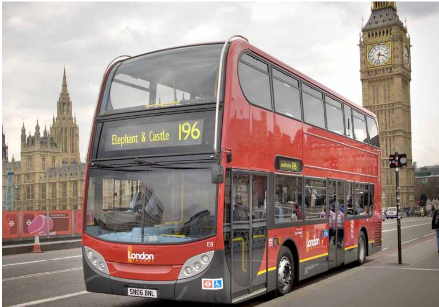
ADL and BAE Systems – their range of hybrid-electric buses are achieving 35 per cent fuel and CO 2 reductions
